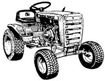
Model B-80 8 speed, 8 h.p. with 36" Mower attachment
