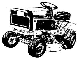
36" mower and 5-bushel rear mounted grass catcher cuts and cleans in a single pass on a compact Simplicity Regent Lawn Tractor.
