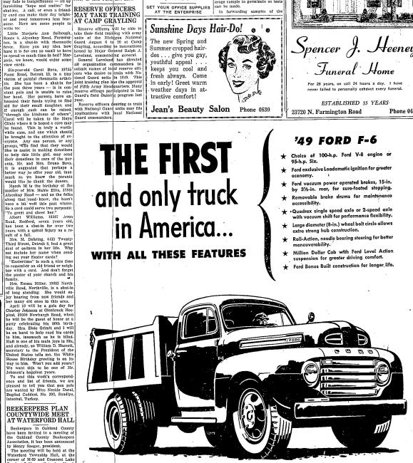
Ford Model F-6 shown. Gross Vehicle Weight rating, up to 15,500 lbs. with 8.25-20 lires. When used as trador, gross combination weight rating, up to 28,000 lbs.
