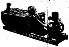
THE PUMP is solid brass, mounted on a cast iron base THE FUM! is solid brass, mounted on a cast-iron base. The valves, which are brass-ball valves, can be removed and replaced by the unscrewing of a single nut. The plunger is solid brass, packed with the best asbestos packing. A repacking nut at the end of the plunger cylinder makes it very easy to repack the plunger. The brass plunger rod is guided by a sliding cross head, running on milled ways.
