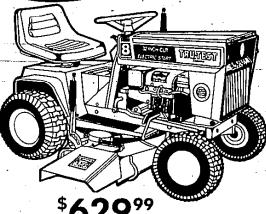
8 H.P. Elec. Start, Synchro Balanced B & S Engine, Gas Gauge, Lo-Tone Muffler, Safety Key Shut-Off, 12 Volt Battery w/Alternator, Floating Front Suspension on Channel Frame, Geared Steering, 13" Front, 16" Rear Wide Pneumatic Tires, Transaxle Drive, 3 Forward—1 Reverse w/Safety Interlock, Disc Brakes, Cigarette Lighter, Ampere Meter, Headlights, Hi-Back Seat, 32" Twin Blade Fully Baffled Floating Deck, Blade Clutch w/Safety Fast Stop Hand Lever, Oversized Chrome Hub Caps. 3-832DE4
