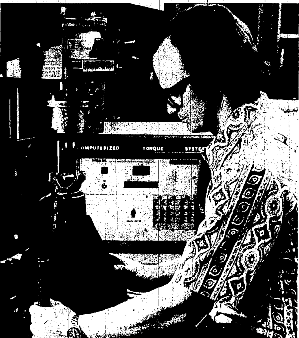
At this work station, a pinion gear pre-load on a differential gear assembly, the DMC-200 micro computer at the rear is integrated with the new Generation II TAS torque assurance system and provides constant monitoring of torque.
