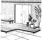
MINI-DECK eliminates dangerous step down from doorsill to patio by leveling walking surface between outdoors and interior floor. Deck is built entirely of Douglas fir 2x4s, with joists laid di-rectly on patio paying Bench by door makes stop-off for trays of refreshments.
