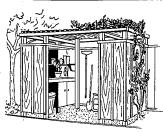
GARDEN STORAGE center built adjacent CANDEN SURACE center built adjacemt to fence gathers outdoor equipment, supplies in central location, with potting shed on one side, storage shelves, cabinets on other. Framing is 4x4-inch posts, 2x4-inch cedar or fir; siding, shelves are western pine. Trellis of 1x2s adds
