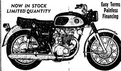
TOP OF THE LINE — 2 Cylinder — 4 stroke. 444cc, 43 H.P. Electric Start, 4-Speed Transmission. Double Overhead Cam Shaft.
