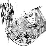
DINKY, PAVED SLAB is expanded to handsome, useful outdoor living area with parquet wood deck. For level yard, dcy. it is laid giver sand and graveb base flush with paving. In sloping land, it's easiest to mount deck on a paving. In sloping land, it's easie post-and-beam frame. Douglas fir lumber is used; shy wood near preservatively treated.
